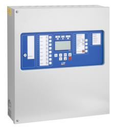
The compact Fire/Extinguishing Control Panel BC08 has been designed for use in single-zone extinguishing systems. Proven conventional technology allows the connection of automatic fire detectors, manual call points and contact detectors.
